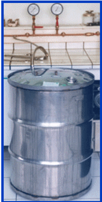
Air pressure test
